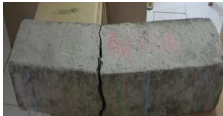
Fig.10: Failure of Singly Reinforced Beam
