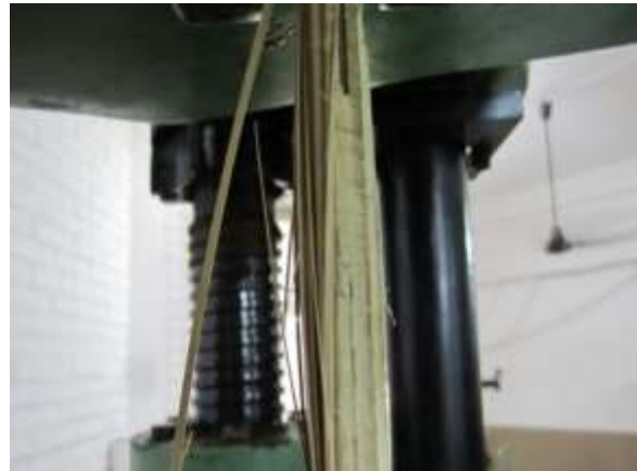
Fig. 3: Failure of the Bamboo Specimen in UTM
