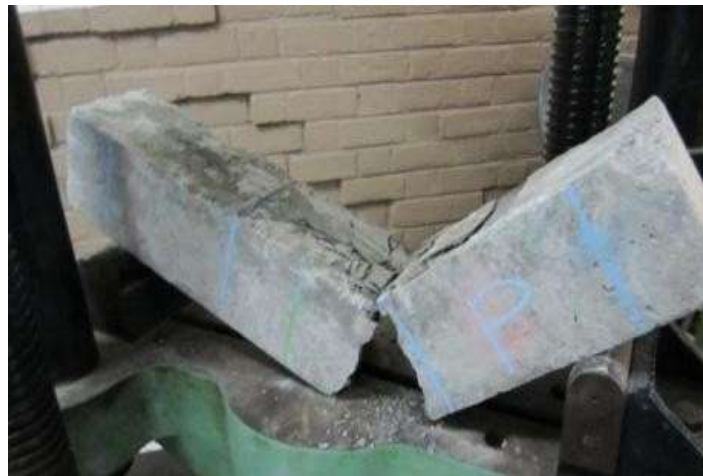
Fig.7: Cement Concrete Beam Failure
